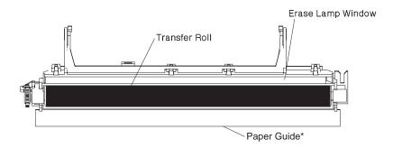
\* Transfer roller housing for 10P has no paper guide
